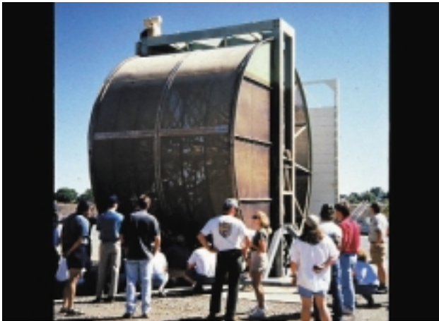
Figure 6. Rotary drum screen (large drum screen, 19' in diameter; Red Bluff, California)
