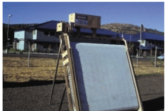
Figure 8. Traveling belt screen (plastic; 10 cfs solar powered screen; eastern Oregon)
