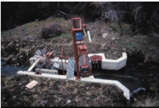
Figure 3. Rotary drum screen (self-cleaning single drum screen; paddle powered; one-bay; John Day River Basin, eastern Oregon)
