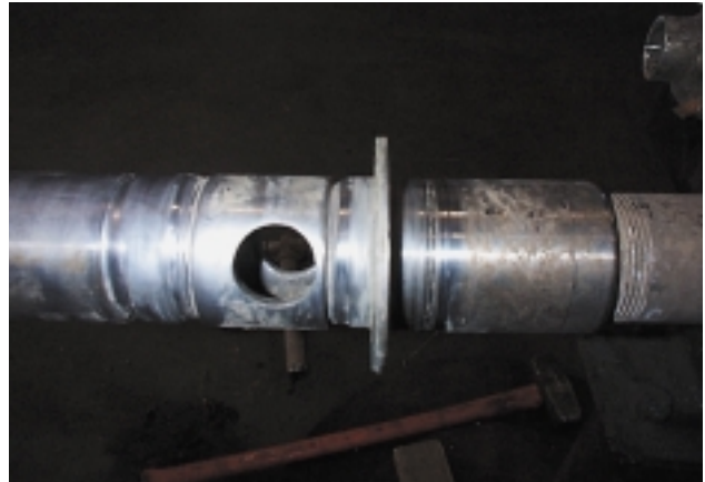
Figure 17. Grit damage to the screen cleaning system
