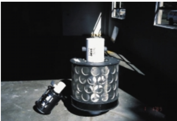
Figure 12. Sure-Flo pump screen (self-cleaning pump screen; water velocity balance tube inside)
