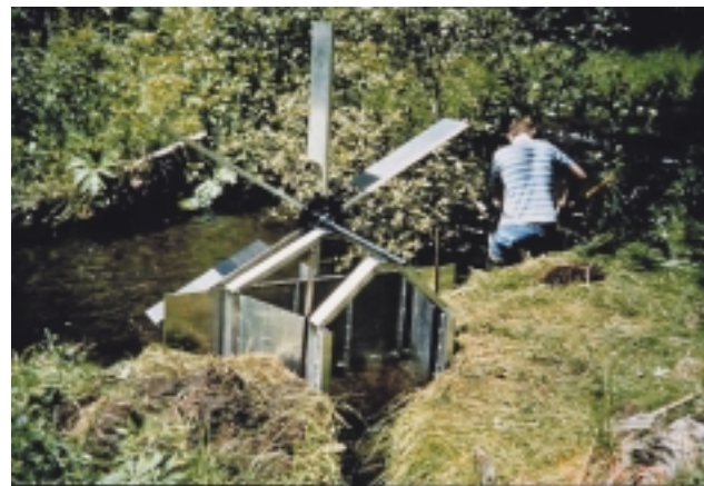
Figure 2. Paddle box screen (screen at ditch diversion point in Jack Creek, eastern Oregon; stream powers paddle; brush on one paddle cleans screen; 1 cfs)
